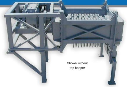
The Barclay 2S Secondary Shredder is a top feed shredder designed to further reduce tire pieces produced by Barclay Primary Shredders. With cascading blade sizes ranging from 2.00 to 1.60" thick, this machine will produce chips for tire derived fuel or granulating. Top feeding allows oversized pieces to be re-fed.
