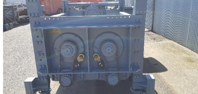
The 4.9 Top Feed has a cut width of 4.9" and a total of 288 blades and bases. Rotating stripper between the rotors prevent material from becoming stuck inside the shredder or wrapped around the shaft.
