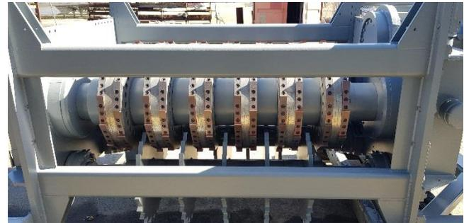
The shredder is powered by a helical bevel "C-Face" motor and gearbox. The motor is controlled with a soft start control system enclosed in an electrical panel. It can be wired to accommodate a wide range of voltage/hertz ratios. Whether you are doing single pass shreds, reshredding, or are looking to increase processing volume, the Barclay 4.9 Top Feed is a great solution.
