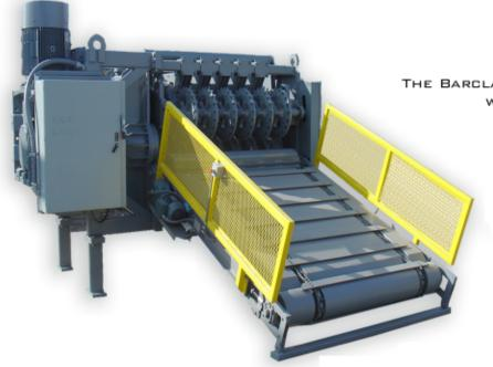
THE BARCLAY 4.9 PRIMARY SHREDDER WAS DESIGNED WITH THE PURPOSE OF BEING THE FIRST AND FOREMOST CUT IN ANY SHREDDING LINE. IT IS CAPABLE OF CUTTING RIM FREE TIRES RANGING IN SIZE FROM PASSENGER TO SUPER SINGLE TIRES.
